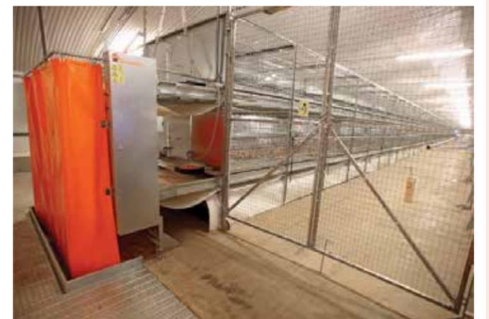
Efficient manure removal is an integral part of the system. In Germany, tight ammonia controls make it difficult for a producer to rear pullets without constant manure removal in place. But it is also to the benefit of bird health, the better environment cuts incidence of burns and blindness in pullets.
