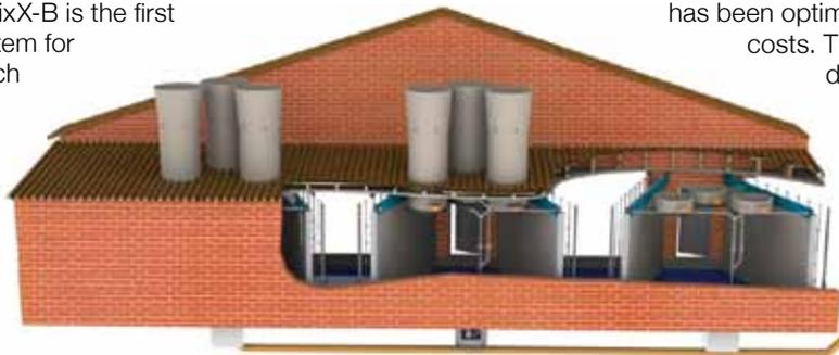
Schematic diagram of the MagixX-B exhaust air treatment system from the rear side
