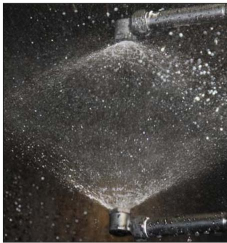
Special arrangement of the nozzles for a high separation of dust and  $\text{NH}_3$
