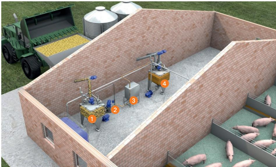
**PEF** stands for **Pulsed Electric Fields**. High-voltage pulses are applied to the chopped maize plant, making it digestible for pigs.
